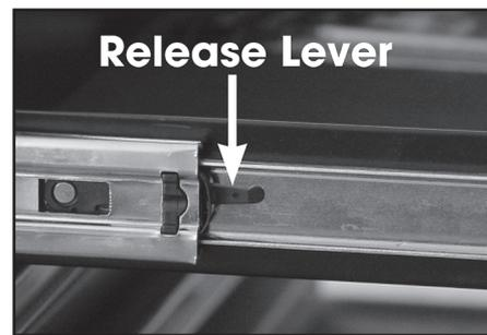
2. With levers pressed as described in step 1, pull drawer from Tool Storage Unit.
